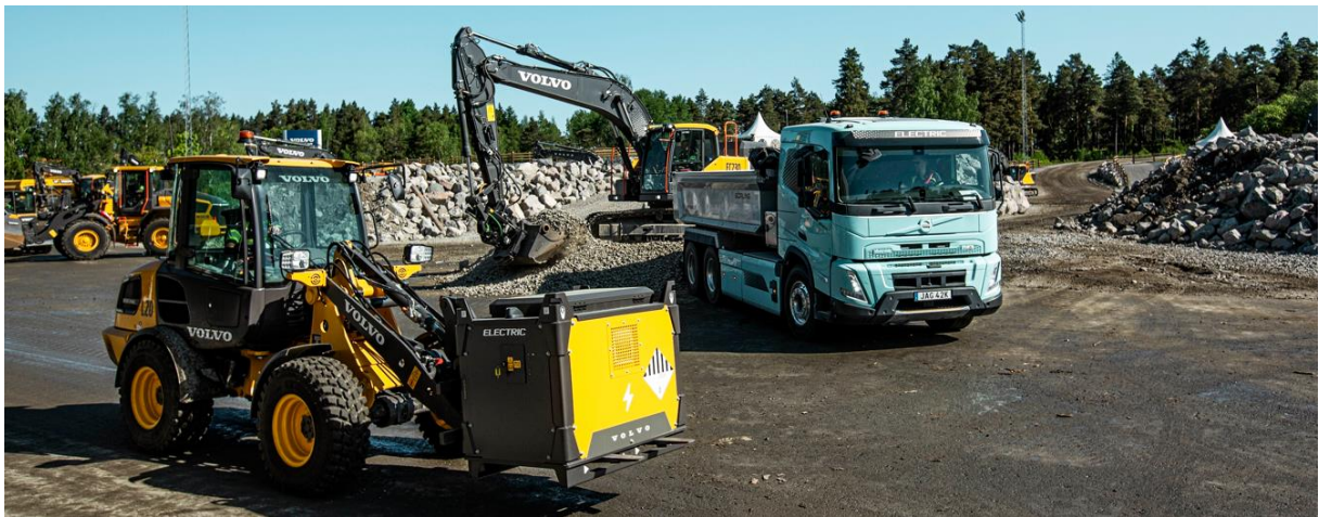
The PU40 power unit is one of a variety of flexible charging solutions.
