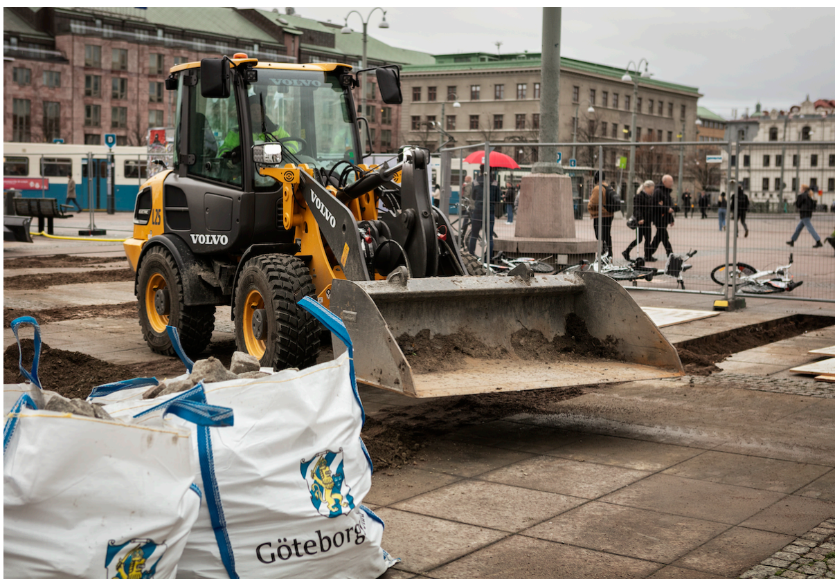
The L25 Electric compact excavator working at Drottningtorget in central Gothenburg. Photo: Electric Worksite.
