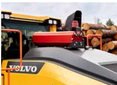
Fire Suppression System
