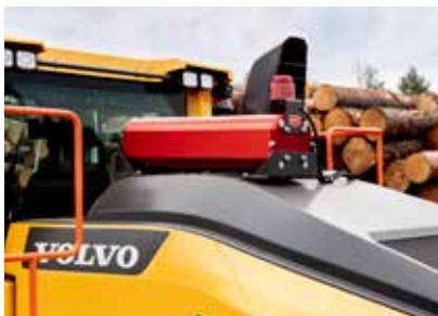
Fire Suppression System
