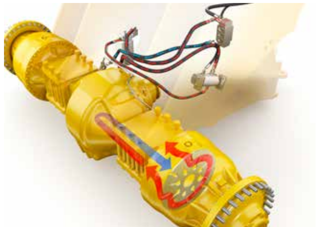
External axle oil cooling
