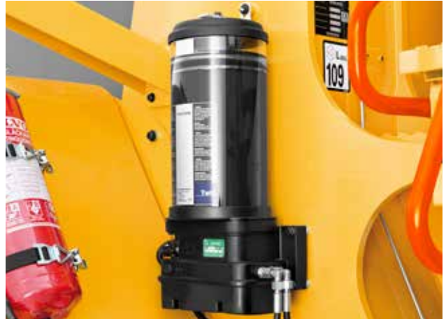
External axle oil cooling
