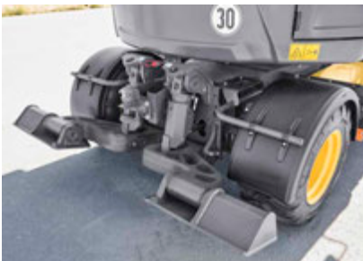
In-line outriggers with trailer hitch
