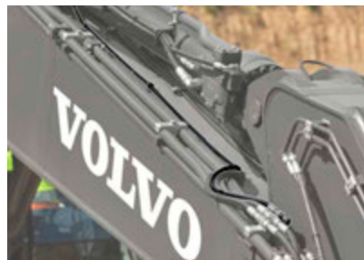
Oil drain line
